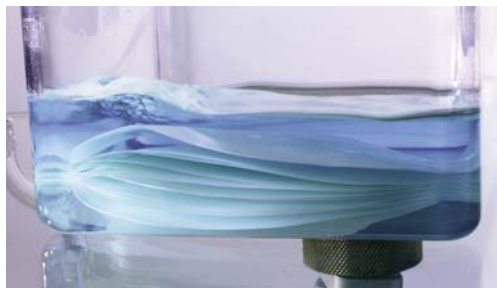
The unique motion of the Belly Dancer produces this unexpected efficiency: separation and thorough washing of multiple filters in a single container.
